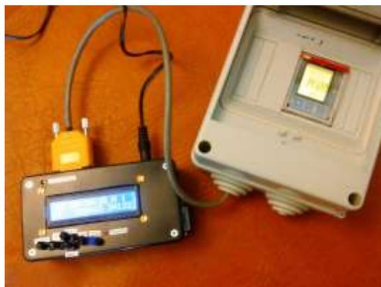
Figure 2.2. The completed datalogger reading the kWh register of a connected meter.
